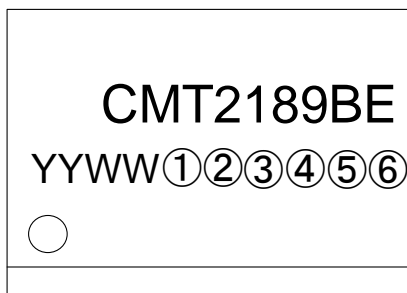
Figure 6. CMT2189BE Top Marking
