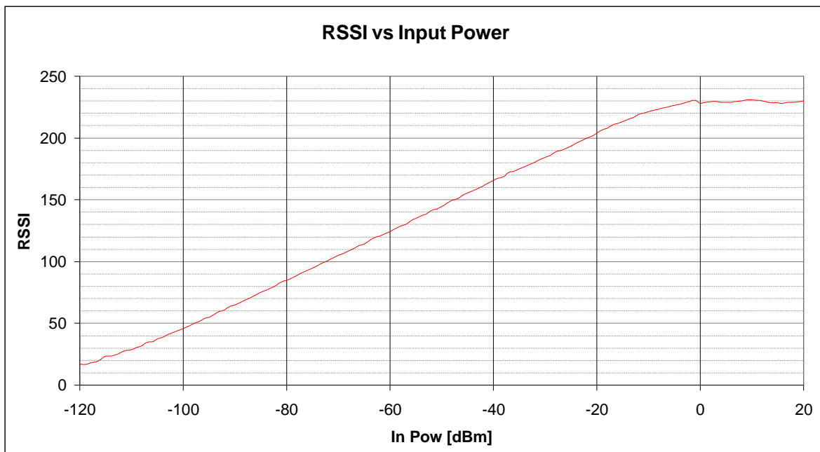
Figure 23. RSSI Value vs. Input Power
